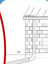
Extend Downspouts and Sump Discharge Pipes at Least 2m from Foundation
