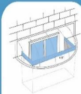
Install Window Wells that Sit 10-15 cm Above Ground and Upgrade to Water Resistant Windows
